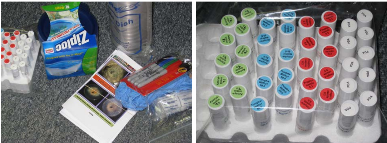
Figure 1. The Profile resistance testing kit contains petri dishes, toothpicks, a scalpel and replacement blades, one lighter, a box of nitrile gloves, four permanent markers, parafilm, lip balm tubes, and a user's manual. The lip balm tubes contain potato dextrose agar and are either impregnated with fungicides at discriminatory doses, or in the case of the control, are purely agar.
